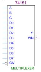
27. In class, we implemented a full-adder using a 3:8 decoder and two OR gates. For this question, implement a full-adder using two 74x151s.
